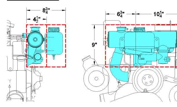
Before purchasing this system, make sure there is enough room in the engine compartment to accommodate the heat exchanger, expansion tank, and necessary components.
