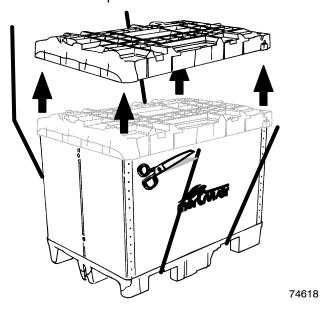
2. Remove the four metal corner posts and place in underside of top cover. Turn latches to lock posts in position.
