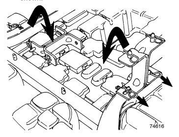
Position folded sides of container on base. Place top cover over base assembly. Stack no more than four complete assemblies together and band for shipping.
