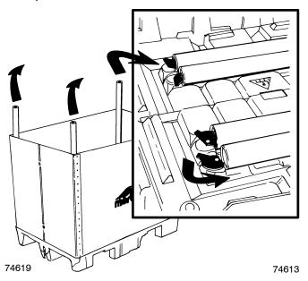
3. Remove the sides of the container and fold flat as shown. Place aside temporarily.
