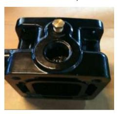
• Tighten the anodes following the same procedures as the anodes placed in the manifolds.
