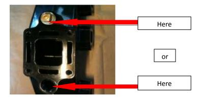
• Tighten the plug until it is tight. This is done with a wrench. Note: The threads won't always bottom out or sit flush with the manifold. Over
