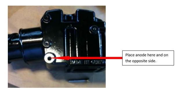
Tighten the anodes following the same procedures as the anodes placed in the manifolds.
