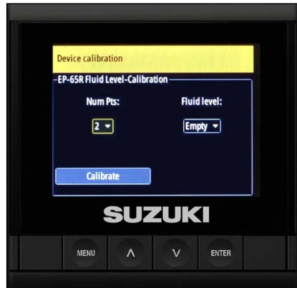
4. Select **Empty** from the **Fluid level** drop-down, then select **Calibrate** and press **Enter**.
