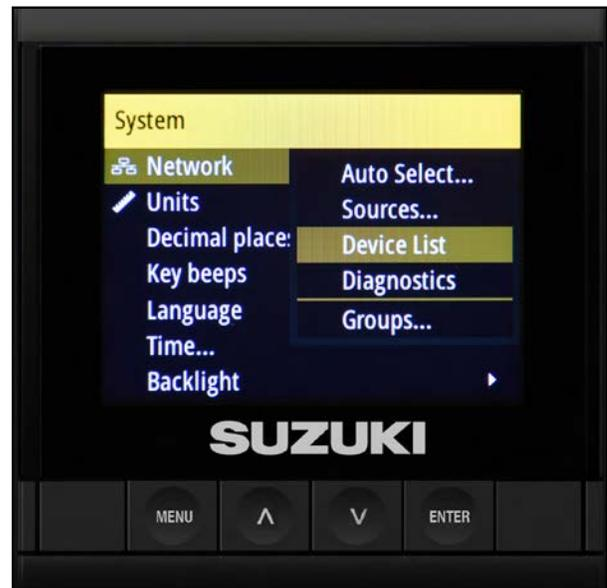
6. The Device List screen that opens is used to access and configure each device connected to the network.
