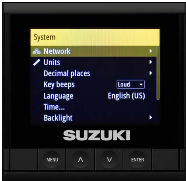
4. A message advises you that this screen re-selects and removes any invalid data source selections, to make sure that all network devices are connected and turned **ON**. Then select **Yes** and press **Enter**.
