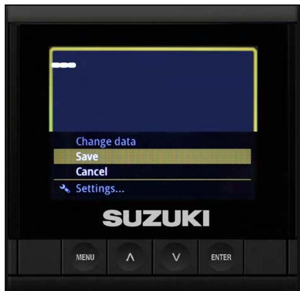
18. After adding the custom page, the data is saved and the operator can scroll through the three default pages and the custom page that has been added. For example, the fuel remaining screen.
