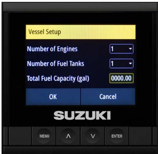
2. Use the arrow buttons to set the fuel capacity and press **Enter**.
