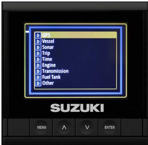
14. Press the down arrow button to select **Fuel Tank** and press **Enter**.
