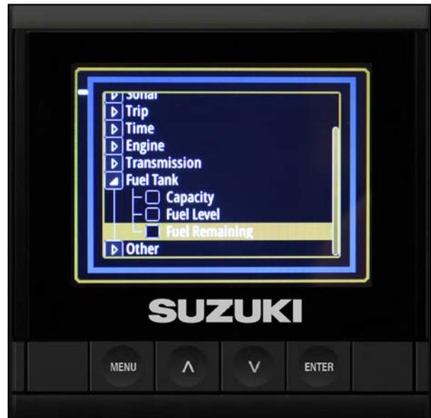
16. After selecting the data, the screen highlights the frame of the C10 Color Display.
