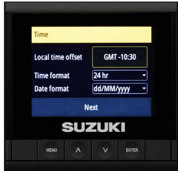
1. To set the time and date manually, use the arrow buttons to select **Time format**, then use the arrow buttons to select the 12-hour or 24-hour time format and press **Enter**.
