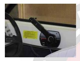
1.1 (Above) Put the boat into forward gear. Trim the sterndrive down.
