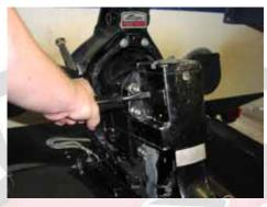
1.3 (Above) Remove the upper plug. This will help it drain faster. Replace both plugs after it has drained.
