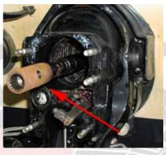
3.2 (above) Check engine alignment with the engine alignment tool. If you do not own a tool, you can take it to a repair shop to get it checked.
