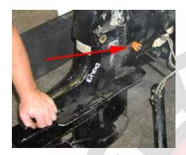
2.5 (Above) Once all the nuts are off you should be able to pull the sterndrive straight back. If it is not moving you can place the handle of a large screwdriver between the upper case and the gimble ring and push on the back of the sterndrive to pop it loose.
