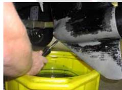
1.2 (Above) Place a suitable container under the bottom drain plug. Remove the bottom drain plug.
