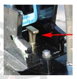
3.5 (Above) Put the sterndrive into forward gear. To do that simply turn the brass shift shaft clockwise, while turning the propshaft counterclockwise.
