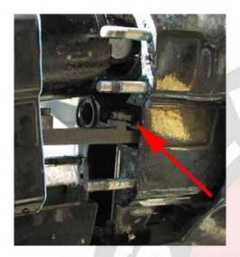
3.7 (Above) As you bring the sterndrive into position, make sure that the shift slide stays engaged to the roller and goes into the upper housing straight. It may be easier with 2 people.
