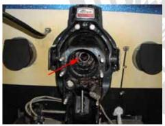
3.1 (Above) Rotate the gimble bearing by hand. If it feels smooth it should be okay. If it is rough at all it should be replaced.
