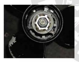
3.8 You may need to rotate the propshaft counterclockwise as you push the sterndrive on. It will aid in lining up the splines. It is best if you have the prop installed, it will give you something to grab onto. Now install the washers and nuts that
