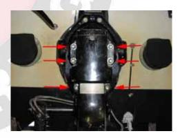
2.4 (Above) Remove the six 5/8 nuts that hold the sterndrive to the bellhousing.
