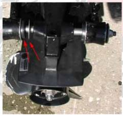
4.2 (Above) Install the washers and inside bushings on the pins.
