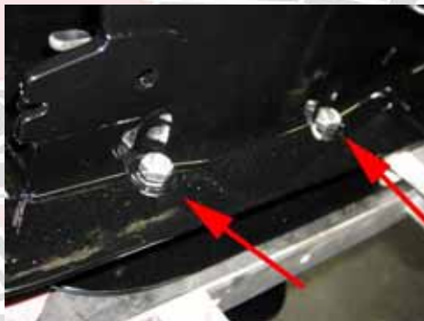
1.4 (Above) Remove the four bolts and nuts. There are two on each side of the Drive. You will need two 5/8 wrenches to remove them. Once those are off you can separate the upper from the lower. It may be necessary to pop the halves loose. Use a rubber hammer or some other soft tool.
