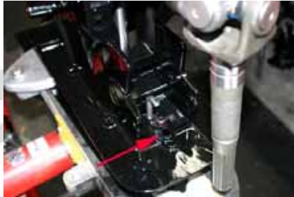
1.3 (Above) Remove the front bolt. Use a 1/2” wrench or socket.
