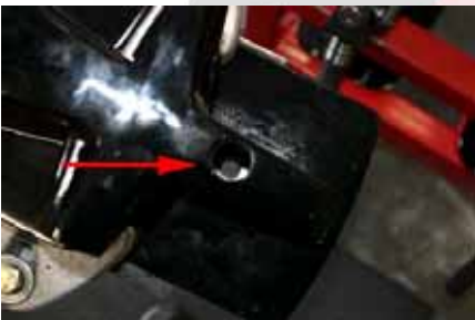
1.1 (Above) Remove the trim tab bolt with a 1/2” socket.
